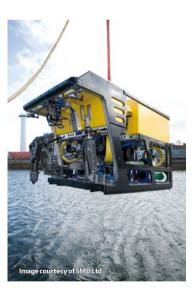
Eccofloat® TG range of syntactic foams are lightweight for building manned and remote operating vehicles. The foams are also used to manufacture mine neutralization systems because of their zero magnetic and sea-water comparable acoustic signatures. Applications include hydroplanes, rudders. trim adjustment modules for submarines and specialized applications such as acoustic windows due to the material profile and ability to significantly improve sonar functions.
